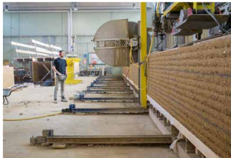
Machine fabrication of rammed earth elements. Photo: Emmanuel Dorsaz
